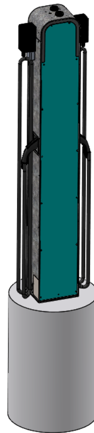
Minimum Pier dimensions: 24" diameter x 36" deep
